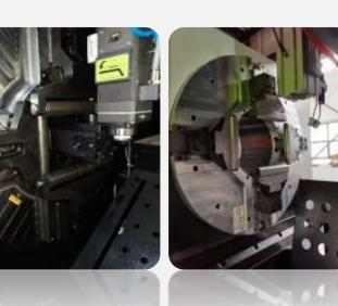
No need to adjust the jaws to replace any shape of pipe
